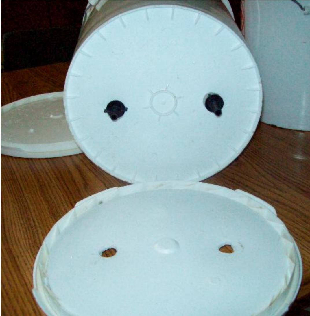
When drilling the bottom of the TOP pail be sure to place it on the top of the lid that will be on the bottom pail this way you will drill both holes at the same time and they will be sure to match up with the drain spouts that come off the filters. Drill two ½” holes like we show here.
