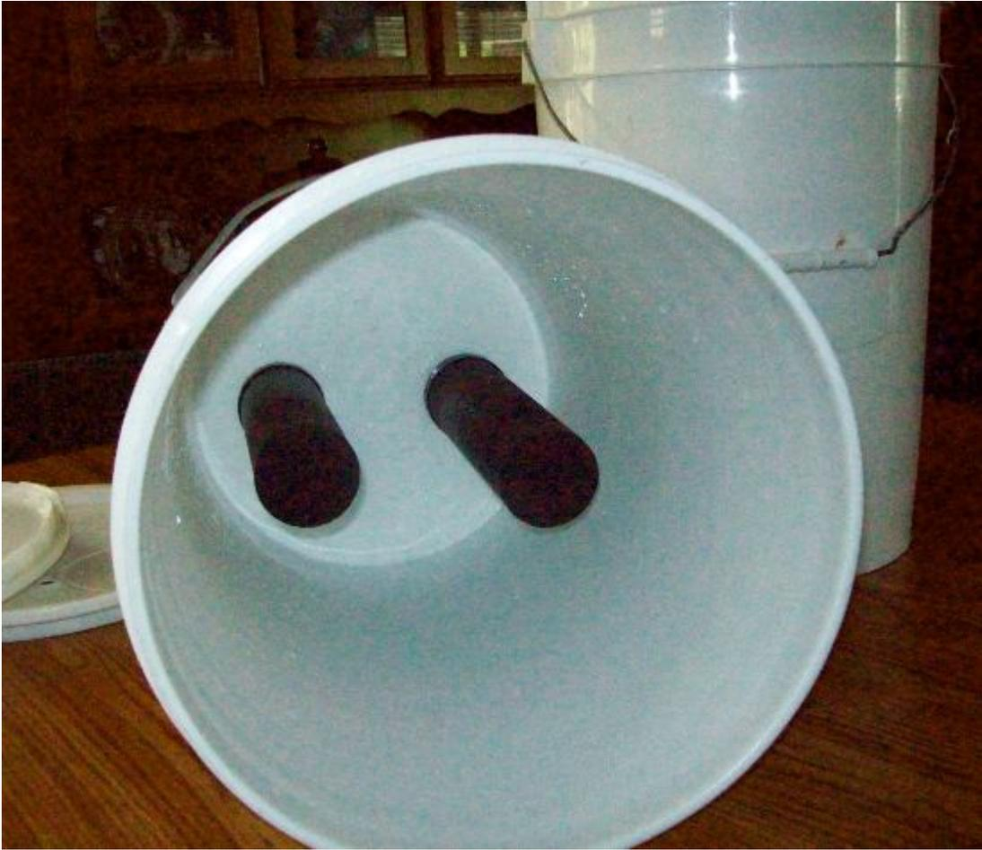
Now install the filters in the bottom of the TOP pail, we choose the Berkey filter but you can use the Ceramic filter just as well. Be sure to put a washer between the filter and the bottom of the pail and then tighten the wing nuts snug but not too tight, remember these are plastic fittings.
