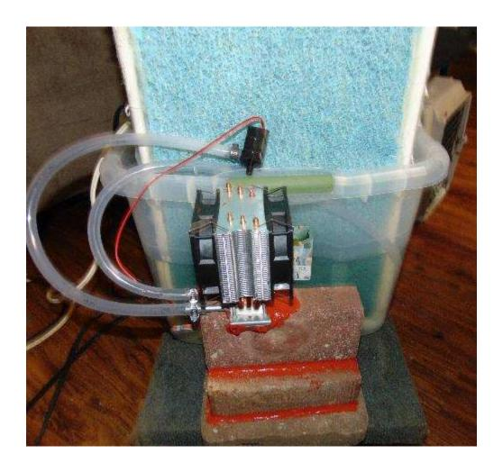
Above shows one Peltier cooler installed with the mini water pump.
